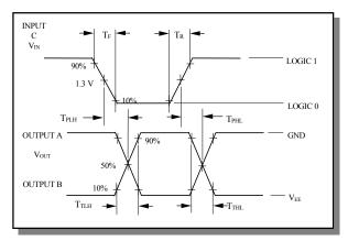
Note: See Switching Wave Forms for the definition of the switching terms. Supplies must be by-passed with .01  $\mu F$  Capacitors
